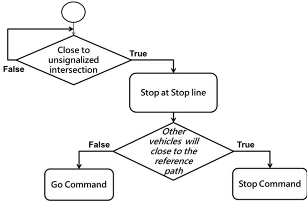
Fig. 3. Architecture of human-like decision model with intention for unsignalized intersection
