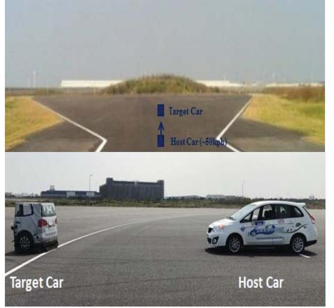
Fig. 1. Scenario 1: CCRs experiment. The top panel illustrates the global view, while the bottom picture presents the side view. The rear one indicates the host car, and the front one represents the target car.
