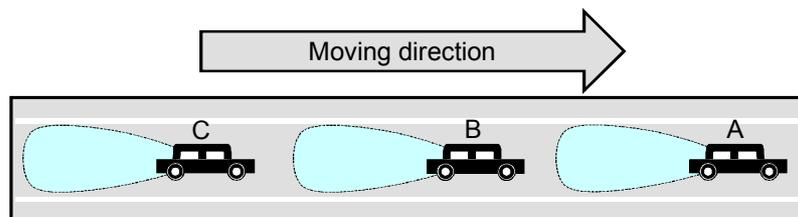
**Figure 3 - Illustration a V2V broadcast through directional antenna**
