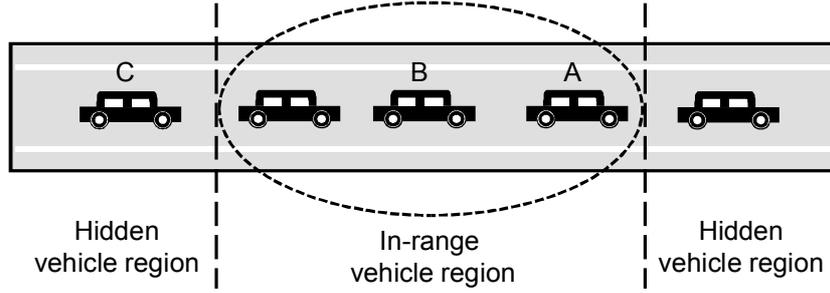
**Figure 1 – Illustration of hidden and in-range vehicle regions relative to centre vehicle**
