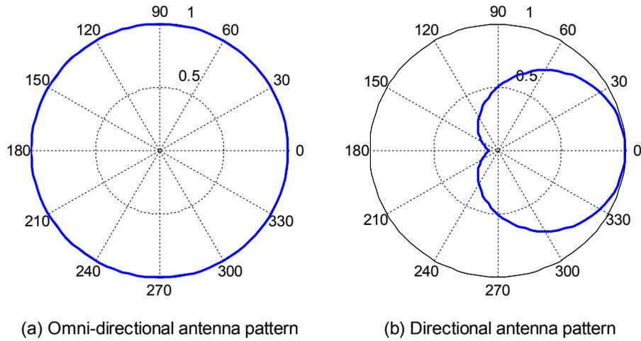
**Figure 2 – Plots of different antenna patterns**
