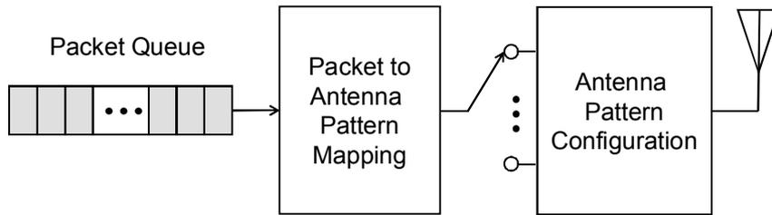
**Figure 4 – Illustration of the proposed adaptive packet transmission scheme**
