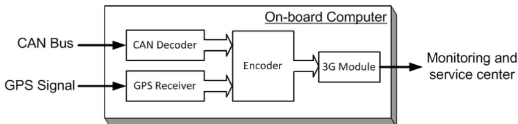
Figure 2: System Block Diagram of On-board Computer.
