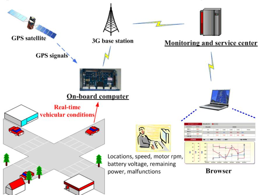
Figure 1: Integrated Framework of the Monitoring and Service Platform.
