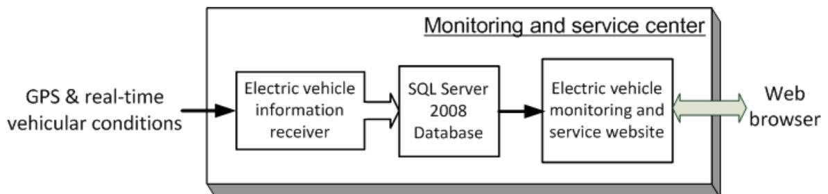
Figure 6: System Block Diagram of the Monitoring and service center.
