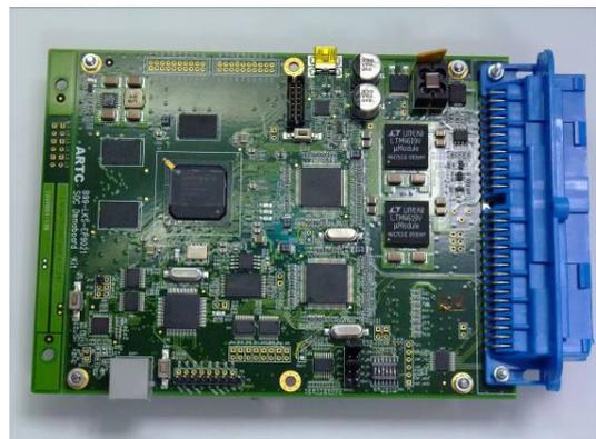
Figure 11 The Xilinx Spartan 6FPGA kit
