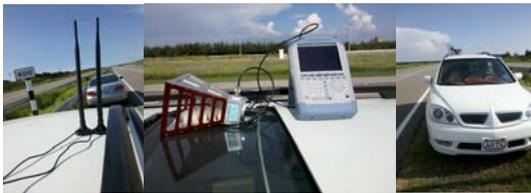
Figure 3: System allocation and horn antenna with analyzer.
