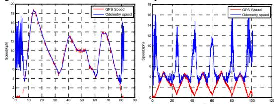
Fig. 10. Gearbox speed test from 0~20 and 0~5kph w.r.t GPS.
