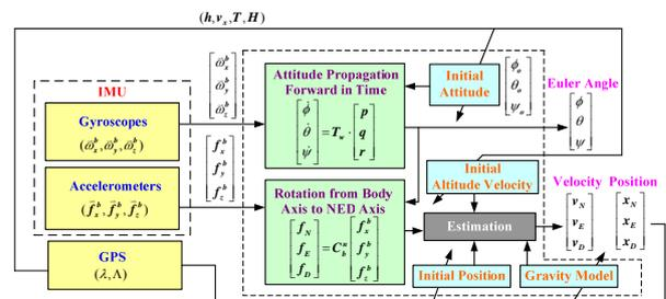
Fig. 6. The block diagram of algorithm in navigation. procedures.
