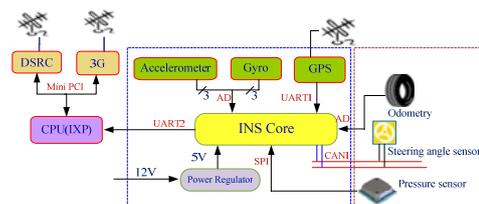
Fig. 3. Block diagram of autonomous platform.
