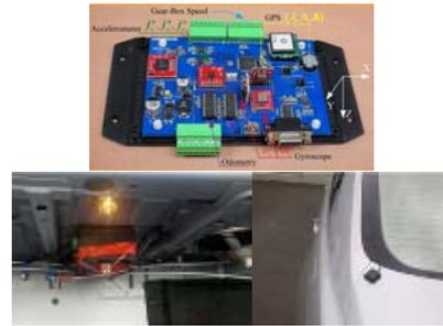
Fig. 2. IMU circuit board which is installed in trunk.
