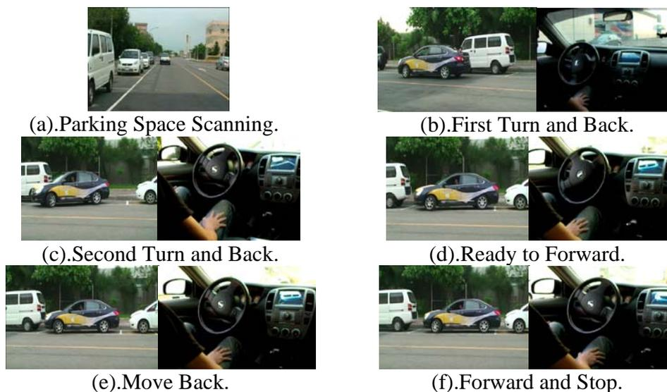
Figure 13(e)-(f): Parallel Parking Test.
