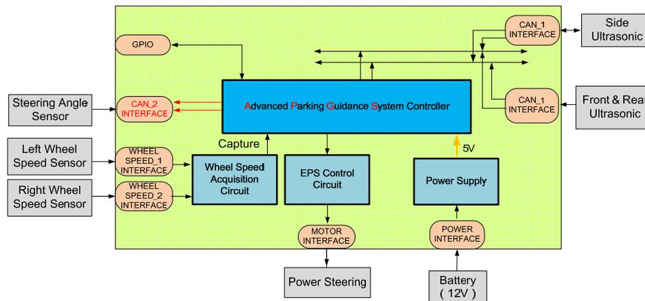
Figure 1: The architecture of advanced parking guidance system.
