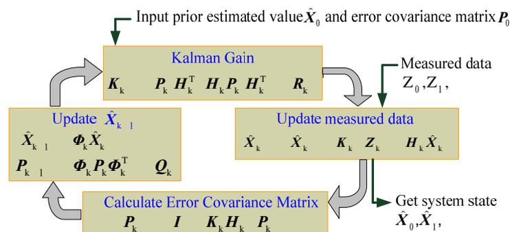
Figure 7: The flow chart of discrete Kalman filter.
