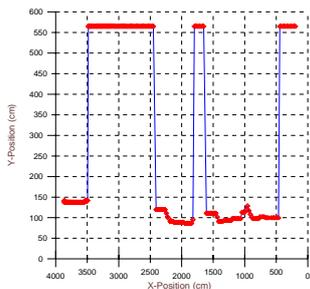
Figure 12: Parking slot scanning.
