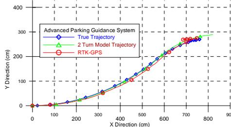
Figure 14: Parallel parking trajectory.
