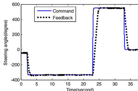
Fig.18. the angle tracking of the type2 control on cement road
