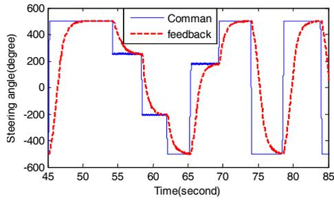
Fig.10. the steering angle tracking performance on asphalt road(type2)
