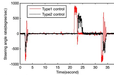
Fig.16. the steering angle rate between different control algorithms
