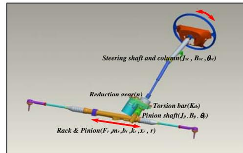
Fig.1. Schematic diagram of an EPS system
