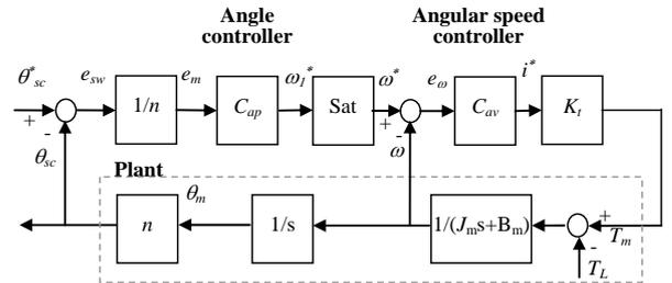
Fig.9. type2 steering angle control algorithm
