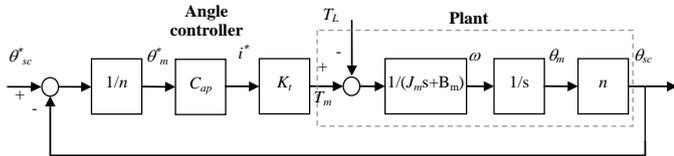
Fig.7. type1 steering angle control algorithm
