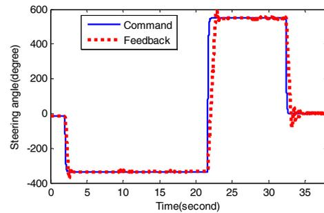
Fig.17. the angle tracking of the type1 control on cement road
