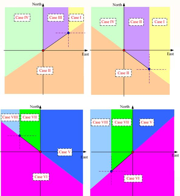
Fig. 3 Collision Conditions with Vehicle A in Quad I to Quad IV.
