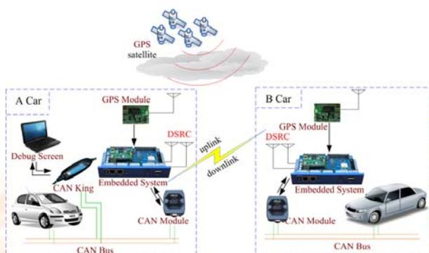
Figure 1 CCW System Architecture
