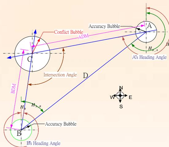
Figure 2 Geometry Model of Two Conflicting Objects.
